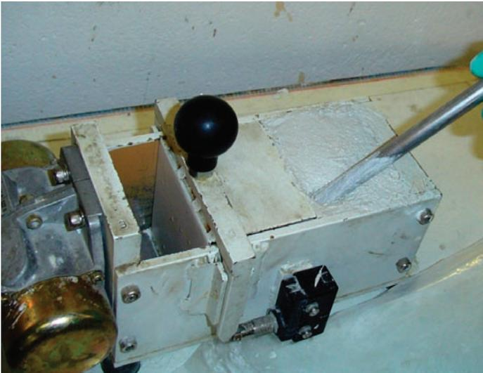
Figure 13: Filling the fluid-meter
